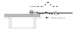
2. Drip Dam(optional) Helps prevent water/rain from running down the antenna wire to the operating position. Squeeze and slide the non-conductive Drip Dam over the open wire end before final insulator install.
